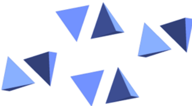
Fig 3. Isolated Si-O tetrahedra in the olivine (\text{Mg,Fe})_2[\text{SiO}_4] structure
