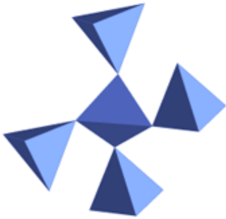
Figure 8. Quartz, SiO 2 . This is a small portion of the quartz structure showing the sharing of all apical oxygens with adjacent Si-O tetrahedra to form a framework.
