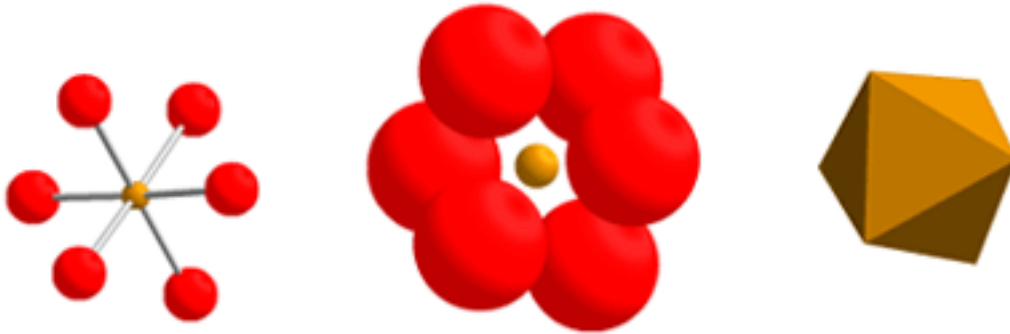
Figure 2. A central iron (brown) atom and six oxygens (red) are shown here in "Ball and Stick", "Space Filling" and "Octahedral" representations. The bonds between the Si and O atoms are shown in gray in the Ball and Stick representation. The relative sizes of the atoms are shown in the Space Filling representation. Note that the size of the interstitial space in the octahedra is much larger than that in the tetrahedra shown above. The brown octahedra represents seven atoms in more complex structures.
