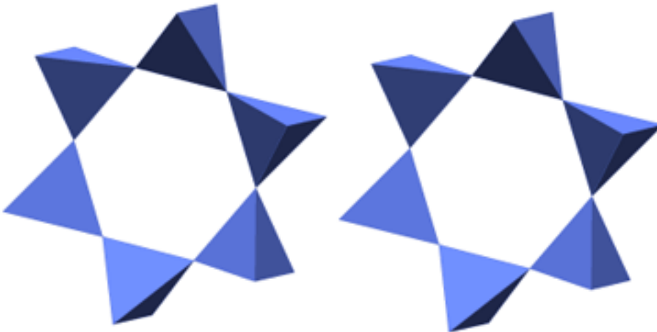
Figure 5. Beryl \text{Be}_3\text{Al}_2[\text{Si}_6\text{O}_{18}] six-membered ring structure. Only two tetrahedral rings are shown.
